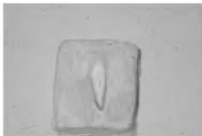
Embedded tooth in plaster slab
